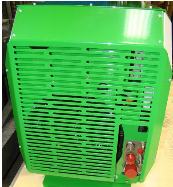
Figure 17. Installing Hydraulics/Electrical Bulkhead Fan End Panel
