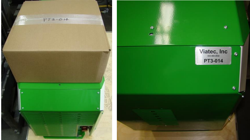
Figure 1. Removing Accessories Box from the Crate
