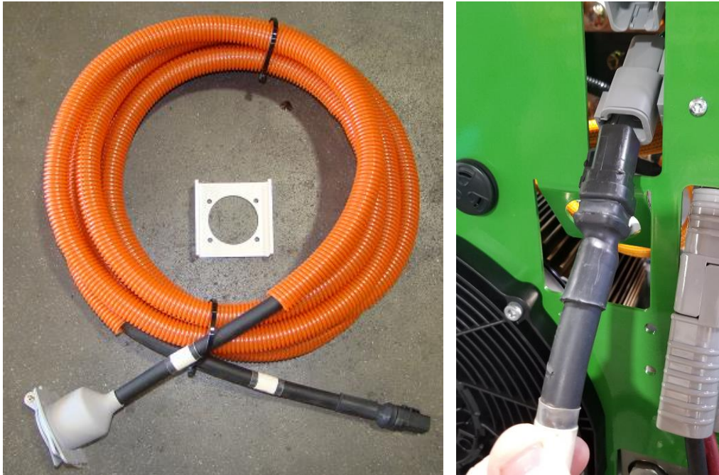
Figure 8. Connecting Standard Charger Harness
