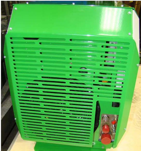
Figure 2. Removing Hydraulics/Electrical Bulkhead Fan End Panel
