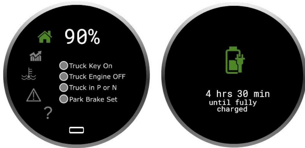
Figure 14. Touch Encoder Home Screen and Charging Screen
