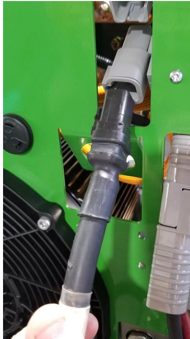
Figure 15. Disconnecting Standard Charger Harness
