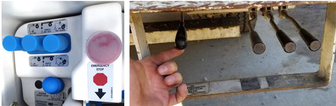
Figure 22. Typical Overhead Boom Operations Panel
