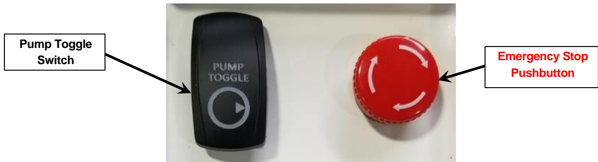
Figure 25. Pump Toggle Switch
