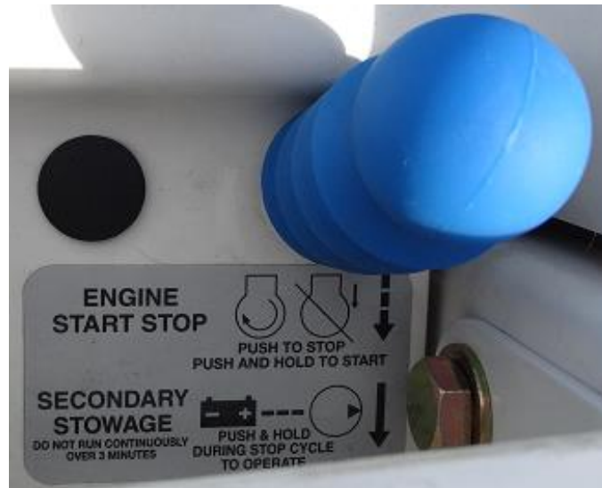
Figure 23. Typical Bucket Mounted Engine Start-Stop Controls
