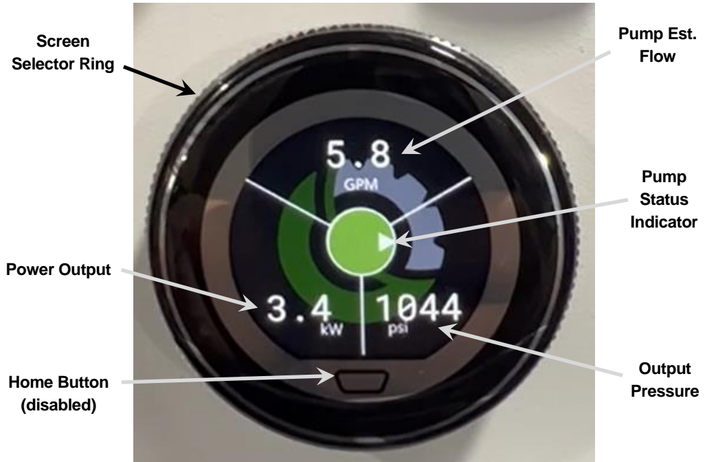
Figure 6. Touch Encoder – Pump Status Screen
