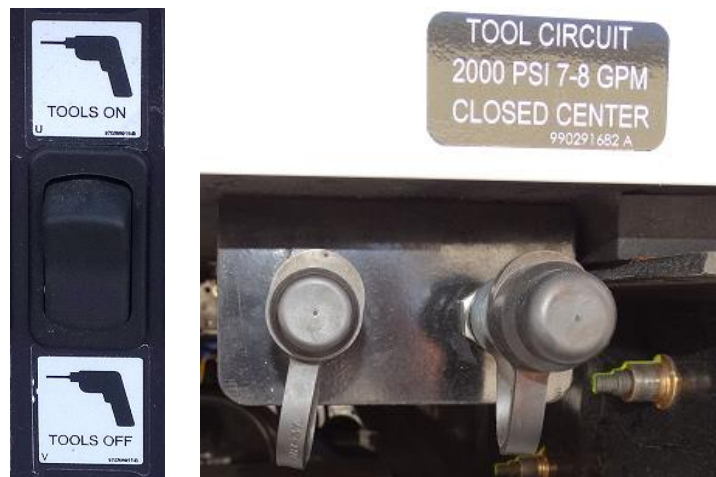
Figure 27. Typical Truck-Mounted Hydraulic Output Panel and Switch
