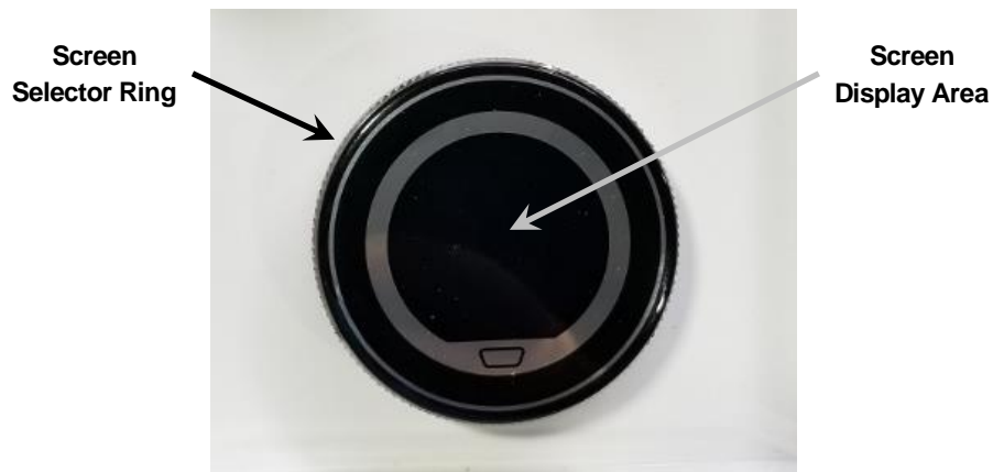
Figure 10. Touch Encoder Screen Selector Ring and Display Area
