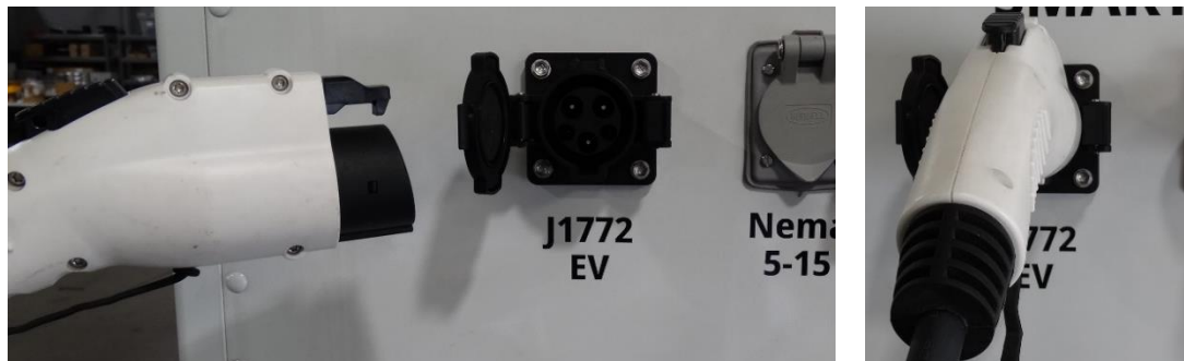
Figure 31. Connecting to J1772 EVSE (Level 2) Charge Receptacle
