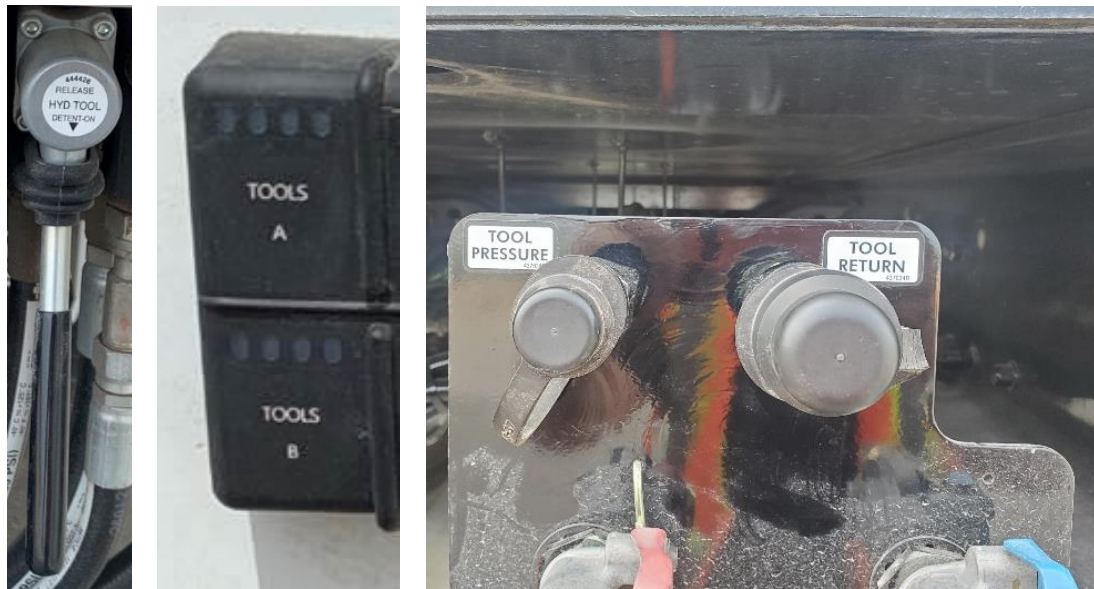
Figure 27. Typical Truck-Mounted Hydraulic Output Panel and Switch
