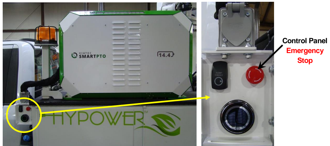
Figure 2. SmartPTO Emergency Stop Location
